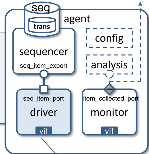
Connection to the DUT is established via the configuration mechanism
