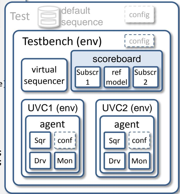
Via the subscribers the expected and the processed transactions become available which are used for the actual checking
